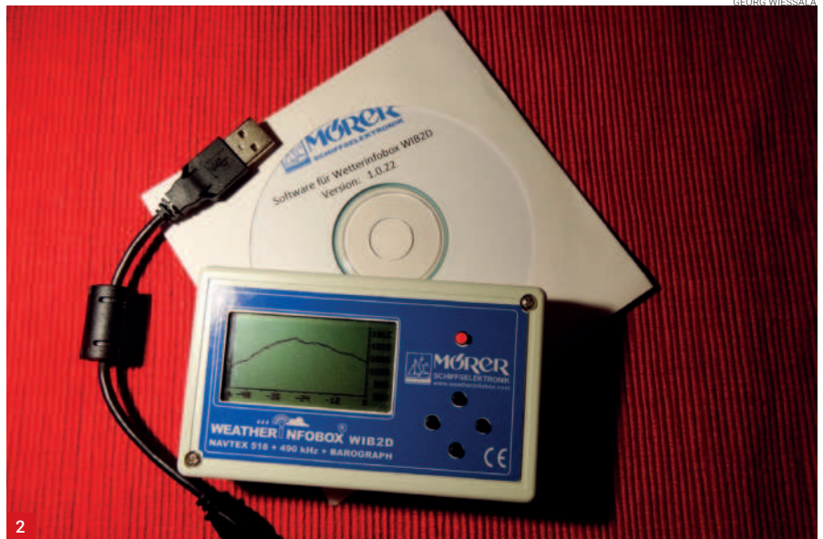
Fig. 1: A GMDSS NAVTEX receiver (L) and marine GPS receiver (R). Fig. 2: The Mörer Infobox WIB2D stand-alone NAVTEX Receiver. Fig. 3: Using Yet Another NAVTEX Decoder (YAND) to decode the messages. Fig. 4: The new NASA Marine BT-3 NAVTEX Receiver for use with your smartphone and the Blue NAVTEX app.
